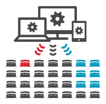
Provisioning is the process of loading a cellular gateway with particular versions of system firmware, application software, and configuration image to prepare the gateway for a specific application or to distribute new features or bug fixes to deployed gateways.
