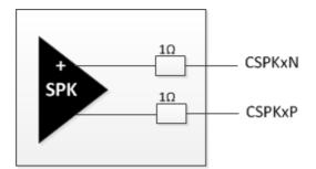
Figure 19. Equivalent Circuit of CSPK
