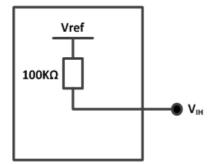
Figure 11. Equivalent circuit of  $V_{IH}$ , Vref > 2.8V
