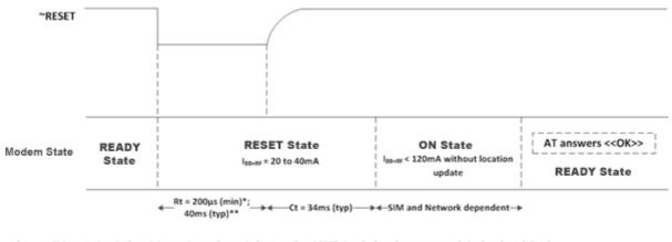
This reset time is the minimum time to be carried out on the "RESET signal when the power supply is already stabilized. •• This reset time is internally carried out by the power supply supervisor only when the modem power supplies are powered ON.
