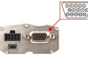
Refer to the following table for the pin description of the 15-pin serial connector.
