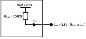
Figure 9. Equivalent Circuit of  $V_{OH}$ , Vref = 2.8V
