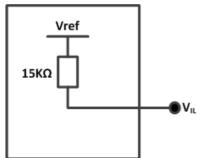
Figure 10. Equivalent Circuit of  $V_{IL}$ , Vref > 2.8V
