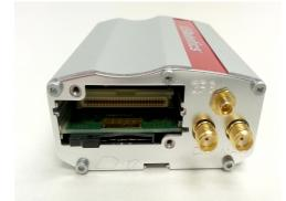
Figure 26. USR3500 expansion compartment
