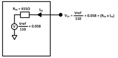
Figure 12. Equivalent circuit of  $V_{OL}$ , Vref > 2.8V
