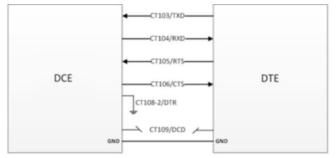
Figure 17. V24 Serial Link Implementation for a 4-wire UART
