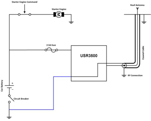
Figure 27. Recommended Power Supply Connection on Trucks
