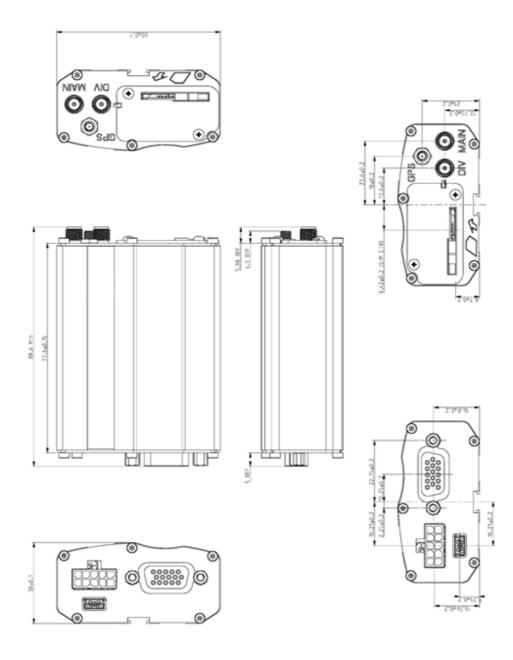
Figure 3. USR3500 Mechanical Drawing
