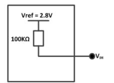
Figure 7. Equivalent Circuit of  $V_{IH}$ , Vref = 2.8V
