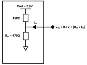
Figure 8. Equivalent Circuit of  $V_{OL}$ , Vref = 2.8V
