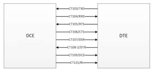
Figure 15. RS232 Serial Link Signals
