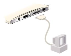
Figure 2-3 Connecting the serial cable
