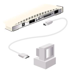
Figure 2-4 Connecting the USB cable
