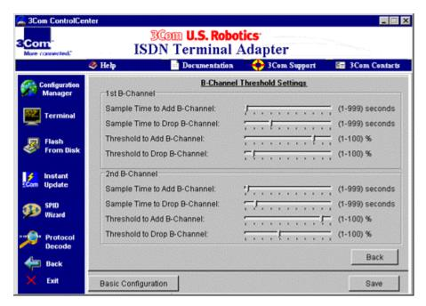
Figure 5-3 ControlCenter "B-channel Threshold Settings" screen
