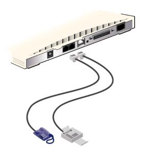
Figure 2-6 Connecting Analog Equipment
