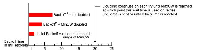
The random backoff used by the access point is a configurable parameter. To describe the random delay, a Minimum Contention Window (cwMin) and a Maximum Contention Window (cwMax) is defined.
