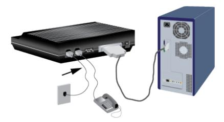
3. To connect a telephone through the modem, plug the telephone's cord into the modem's a jack.
