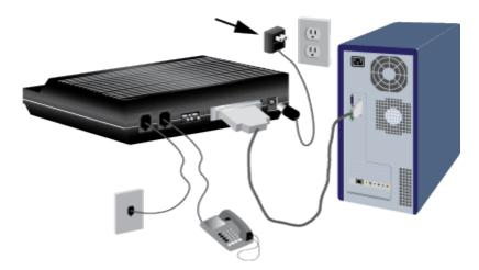
Turn on the modem by switching the power switch on the top of the modem to ON.The CS LED should light.
