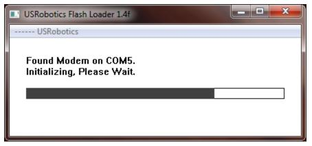
Once the Flash Loader selects the COM port, it will send the file to the modem.
