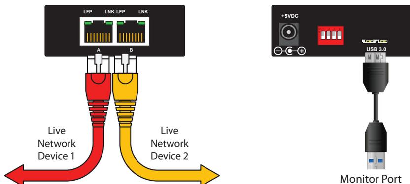
Note: Anytime the configuration switches are changed, remove and then re-apply power for the changes to take effect.
