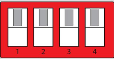
Factory Default Setting DIP 1-4 on: 1 Gig speed, Auto Duplex, Link Failure Propagation on
