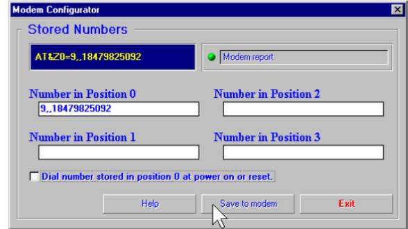
To store a number in your modem’s memory, simply click in one of the entry boxes. Type in the phone number exactly as you would dial it. NOTE: Position Zero has a special feature. You can set your modem to automatically dial this number at Power On or at reset.
