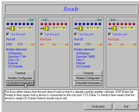
If your modem is installed and configured correctly, Modem Station will find the modem and display make and model information under the assigned port. All currently active ports should display “Port
