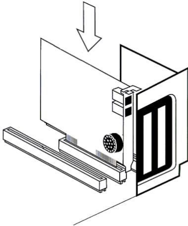
You'll have to apply a little pressure to seat the modem properly. Sometimes a gentle back-and-forth motion helps get the modem all the way into the slot. If you feel resistance, the modem may not be properly lined up with the slot. Do not force it. Take the modem all the way out and try again.
