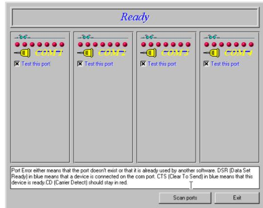
The screen consists of four columns, one for each possible COM port on a PC. You can choose a specific port(s) to scan by clicking the checkbox for that port.
