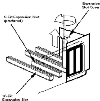
Holding the modem by each corner, align the gold edge with an empty expansion slot. Push down gently until the modem snaps into the slot. (Note: The drawing shows horizontally aligned expansion slots. Some computers have vertically aligned slots. The instructions apply to both styles.)
